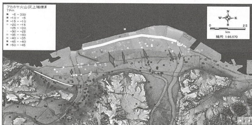
Fig.3 Distribution of upper depth of K-Ah volcanic ash layer, geological structure and area of inferred large displacement
