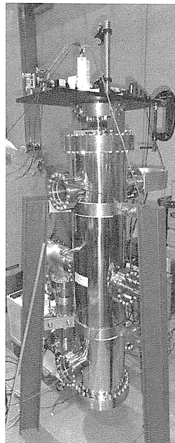
Fig. 1 A photograph of the gravity gradiometer at the ICRR, Tokyo University. The height and weight of the gravity gradiometer are about 1.5 m and 100 kg, respectively.
