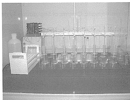
Fig. 1. Schematic description of the semiautomatic system of chemical separation by open column. The solutions (sample solution and eluant) are injected from the test tubes to the open column by peristaltic pump automatically. Changing the test tube and starting the collection of eluate are done manually. procedure.
